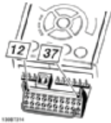
Illustration 5.37: Bridge jumper between terminal 37 and 24 VDC.
