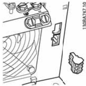
Illustration 5.34: Terminals for relay connections for B3. Only one relay input is fitted from the factory. When the second relay is needed remove knock-out.
