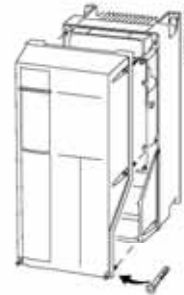
Illustration 5.38: Access to control terminals for A5, B1, B2, C1 and C2 enclosures
