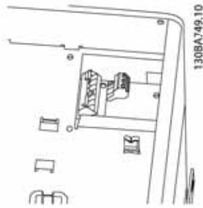
Illustration 5.36: Terminals for relay connections for C3 and C4. Located in the upper right corner of the frequency converter.
