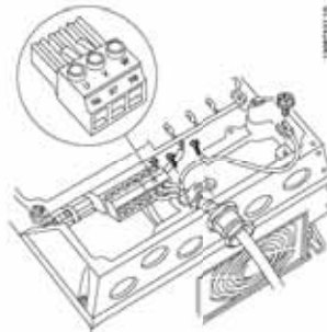
Illustration 5.18: First terminate the motor earth, then place motor U, V and W wires in terminal and tighten. Please ensure that the outer insulation of the motor cable is removed under the EMC clamp.
