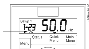
Illustration 7.7 Indicating Motor Direction
