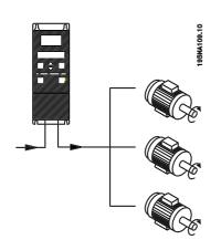
The adjustable frequency drive is able to control several motors connected in parallel. The combined total current consumption of the motors is not to exceed the maximum rated output current ( $I_{INV}$ ) for the adjustable frequency drive. If the motors are to have different rpm values, use motors with different rated rpm values. Motor frequency is changed simultaneously, which means that the ratio between the rated rpm values is maintained.
