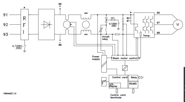
\* Integrated 1A RFI filter and brake is an option. \*\* VLT 2803-2815 200-240 V is not supplied with intermediate circuit coils.
