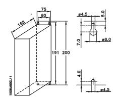
The drawing below gives the mechanical dimensions of VLT 2822 (3 HP) 200-240 Volts and VLT 2822-2840 (3 - 5 HP) 380-480 Volts. All dimensions are in inches.
