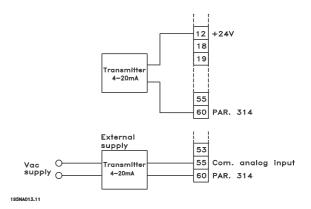
Par. 314 Analog input = Feedback [2] Par. 315 Terminal 60, min. scaling = 4 mA
