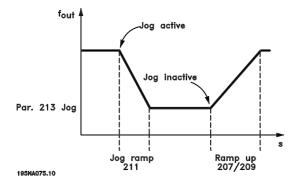
The jog ramp time starts if a jog-signal is given via the LCP control panel, one of the digital inputs or the serial communication port.
