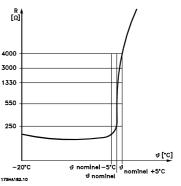
If a motor features a Klixon thermal switch instead, this can also be connected to the input. If motors operate in parallel, the thermistors/thermal switches can be connected in series (total resistance lower than  $3 \text{ k}\Omega$ ). Parameter 128 Motor thermal protection must be programmed for Thermistor warning [1] or Thermistor trip [2] and the thermistor is to be connected between a digital input and terminal 50 (+ 10 V supply).
