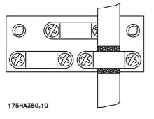
Control wires must be shielded/armored. Connect the shield to the drive chassis with a clamp. Normally, the shield must also be connected to the chassis of the controlling device. (See the instructions for the specific device.) In analog signals or connections using very long wires, 50/60 Hz ground loops may occur because of noise transmitted from the AC line. It may be necessary to break the shield and insert a 100  $\mu$ F capacitor between the shield and the chassis.
