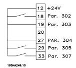
Par. 302 Digital input = Start [7] Par. 303 Digital input = Freeze reference [14]
