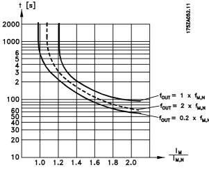
ETR functions 1-4 do not begin to calculate the load until you switch to the Setup in which they have been selected. This means that you can use the ETR function even when changing between two or more motors.
