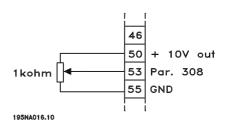
Par. 308 Analog input = Reference [1] Par. 309 Terminal 53, min. scaling = 0 Volt Par. 310 Terminal 53, max. scaling = 10 Volt
