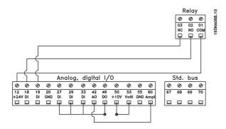
Use the following procedure for the control card test:
