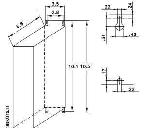
The drawing below gives the mechanical dimensions of VLT 2840 (5 HP) 200-240 Volt and VLT 2855-2875 (7 - 10HP) 380-480 Volt. All dimensions are in inches.
