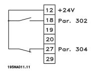
Par. 302 Digital input = Start [7] Par. 304 Digital input = Coasting stop inverted [2]
