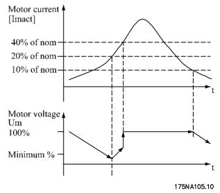
If the active motor current is below 10%, the motor voltage will be decreased by the speed mentioned above until the voltage reaches the setting for Par. 117. If the active motor current comes over 20% the voltage will be increased by the above-mentioned speed. If the active motor current reaches 40% the motor voltage will be increased immediately to normal motor voltage. The reduction in motor voltage depends on the parameter 117 setting.
