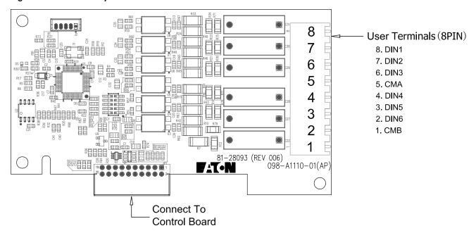
Figure 23. IO5 Board Wire Layout
