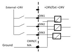
Figure 6. Digital Input Signal Conversion—Negative Logic
