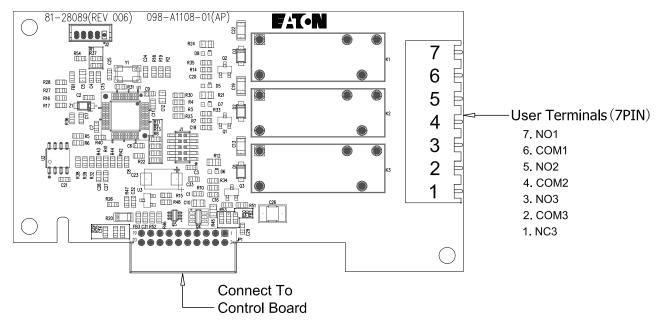
Figure 17. IO3 Board Wire Layout
