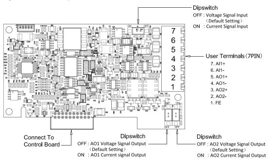
Figure 14. IO2 Board Wire Layout
