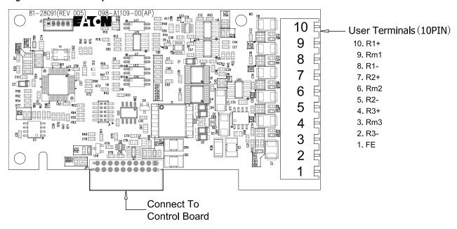
Figure 20. IO4 Board Wire Layout
