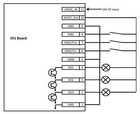
**Note:** If the thermistor inputs are selected, it removes 2 of the digital inputs to be used as the thermistor inputs.
