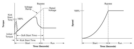
**Kick Start**—The Kick Start feature works in both the Voltage Ramp Start and Current Limit Start modes. By momentarily applying up to a two (2) second pulse of current to the motor, it provides an initial boost in torque to overcome the static friction common in some applications. The level of torque boost is set by the *Kick Start Torq* parameter and the duration of the "kick" is set by the *Kick Start Time*. Setting the *Kick Start Time* to 0 disables this feature.
