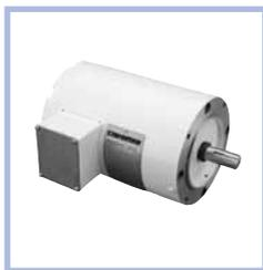
**Applications:** Gear reducers, pumps, fans, blowers, conveyors, and other machinery found in food processing, dairies, slaughter houses, beverage plants, car washes, and other high humidity or wet environments or where motor is subject to high pressure washdowns.
