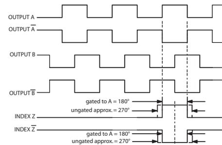
CLOCKWISE ROTATION AS VIEWED FROM THE SHAFT SIDE (FOR UNITS WITH DUAL WHEELS, ORIENT THE ENCODER SO THAT THE LABEL IS READABLE).
