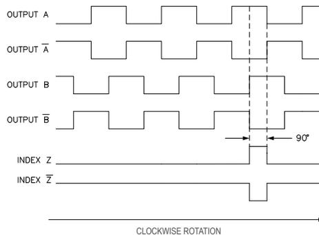
NOTE: ALL DEGREE REFERENCES ARE ELECTRICAL DEGREES. WAVEFORM SHOWN WITH OPTIONAL COMPLEMENTARY SIGNALS A, B, Z FOR HV OUTPUT ONLY.
