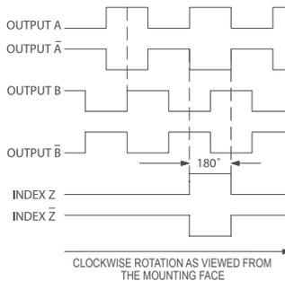
NOTE: ALL DEGREE REFERENCES ARE ELECTRICAL DEGREES. WAVEFORM SHOWN WITH OPTIONAL COMPLEMENTARY SIGNALS  $\bar{A}$ ,  $\bar{B}$ ,  $\bar{Z}$  FOR HV AND H5 OUTPUTS ONLY.
