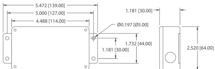
All dimensions are in inches with a tolerance of  $\pm 0.005"$  or  $\pm 0.01"$  unless otherwise specified. Metric dimensions are given in brackets [mm].
