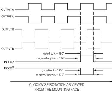
NOTE: ALL DEGREE REFERENCES ARE ELECTRICAL DEGREES. WAVEFORM SHOWN WITH OPTIONAL COMPLEMENTARY SIGNALS  $\bar{A}$ ,  $\bar{B}$ ,  $\bar{Z}$  FOR HV AND H5 OUTPUTS ONLY.
