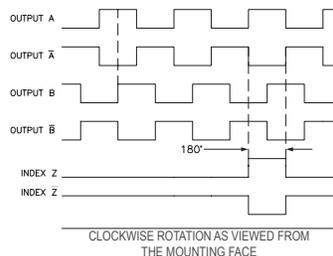
NOTE: ALL DEGREE REFERENCES ARE ELECTRICAL DEGREES. WAVEFORM SHOWN WITH OPTIONAL COMPLEMENTARY SIGNALS A, B, Z FOR HV AND H5 OUTPUTS ONLY.
