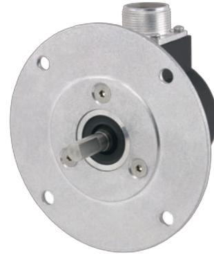
The optional 5PY adapter is made of all aluminum construction and allows the Model 725 encoder to replace DC tachometer technology. The 5PY adapter is mechanically interchangeable with any 5PY tach generator.
