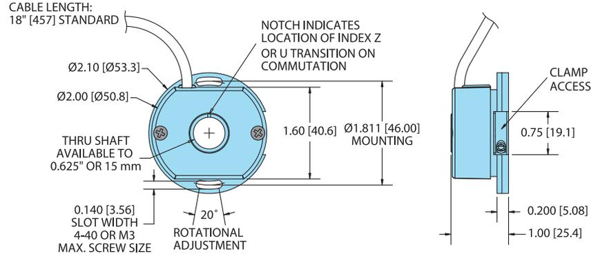
All dimensions are in inches with a tolerance of +0.005" or +0.01" unless otherwise specified. Metric dimensions are given in brackets [mm].
