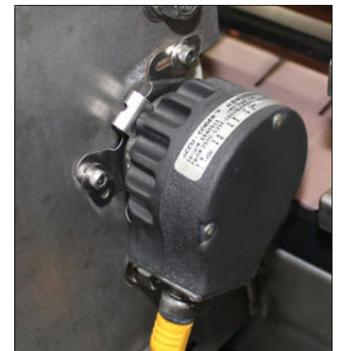
1. **Environmental Seal.** If your encoder will be exposed to dirt, dust and moisture, consider a hollow bore encoder. A thru-bore encoder has two exposed shaft seals that offer potential paths of contaminant ingress. With a hollow bore solution, one seal is protected from contaminants and potential leakage. If the encoder is exposed to washdown or direct water spray, we recommend a hollow bore housing if possible.
