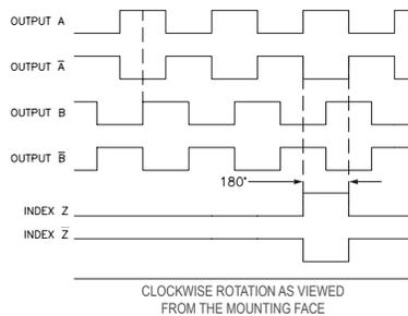
NOTE: ALL DEGREE REFERENCES ARE ELECTRICAL DEGREES. WAVEFORM SHOWN WITH OPTIONAL COMPLEMENTARY SIGNALS  $\bar{A}$ ,  $\bar{B}$ ,  $\bar{Z}$  FOR HV OUTPUT ONLY.
