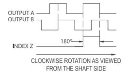
NOTE: ALL DEGREE REFERENCES ARE ELECTRICAL DEGREES. WAVEFORM SHOWN WITH OPTIONAL COMPLEMENTARY SIGNALS A-bar, B-bar, Z-bar FOR HV OUTPUT ONLY.
