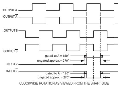
NOTE: ALL DEGREE REFERENCES ARE ELECTRICAL DEGREES. WAVEFORM SHOWN WITH OPTIONAL COMPLEMENTARY SIGNALS  $\bar{A}$ ,  $\bar{B}$ ,  $\bar{Z}$  FOR HV OUTPUT ONLY.
