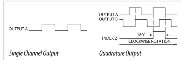
A single channel encoder, often called a tachometer, is normally used in systems that rotate in only one direction and require simple position and velocity information.
