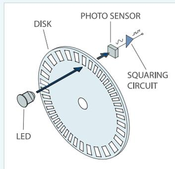
Resolution is a term used to describe the Cycles Per Revolution (CPR) for incremental encoders. Each incremental encoder has a defined number of cycles that are generated for each 360 degree revolution of the shaft. These cycles are monitored by a counter or motion controller and converted to counts for position or velocity control. The diagram shows how the whole encoder comes together.
