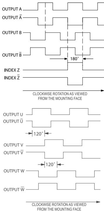
NOTE: ALL DEGREE REFERENCES ARE ELECTRICAL DEGREES. WAVEFORM SHOWN WITH OPTIONAL COMPLEMENTARY SIGNALS  $\bar{A}$ ,  $\bar{B}$ ,  $\bar{Z}$  FOR HV AND OD OUTPUTS ONLY.
