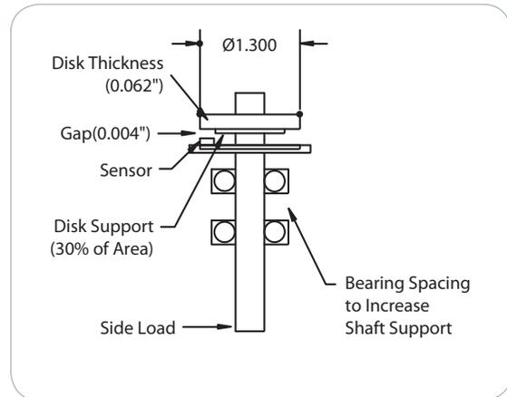
doubled from 0.002" to 0.004", and the disk diameter was reduced from 2.0" to 1.3".
